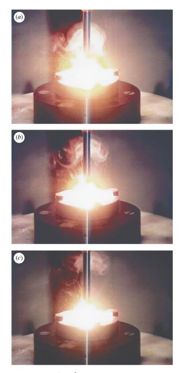
Figure 7. Successive video frames  $(25 \text{ s}^{-1})$  showing the rising incandescent vortex around the top electrode, after a 14 kV pulse discharge on a deep bed of Takahe A soil equilibrated with 100 % RH air (without carbon wick). A water resistor of 100  $\Omega$  was used, with the air gap 15 mm.
