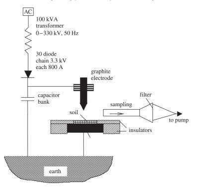
Figure 2. Experimental arrangement showing the power supply, electrode geometry and gas sampling.
